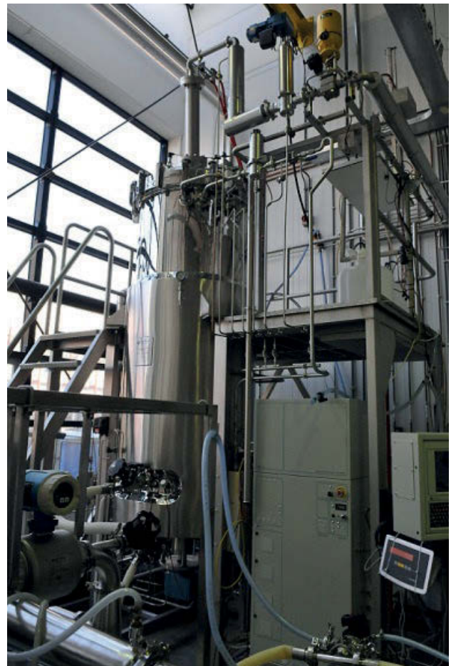
Figure 8 A 1500 litre steel fermenter at Food & Biobased Research, Wageningen UR
